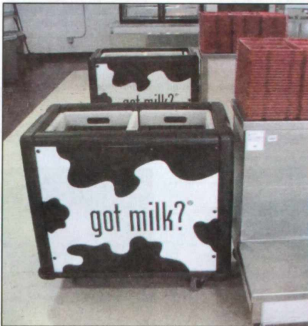
Two new milk coolers with removable inserts that are put into the freezer when not in use.
