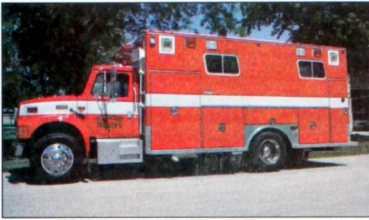
Truck 1880 is a 1994 International 4900 equipment truck. The truck also transports firefighters to the scene of an emergency and can be used as a central command vehicle.
