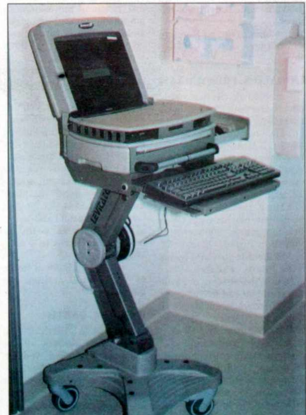
Moving into the 21st century was a big part of the move to the new hospital campus according to Janet Ford, Public Relations Director for the hospital. Shown above is what is known as a COW, computer on wheels. The COWS will be used for each patient and takes the place of the manual clipboards used previously to track patient information.
