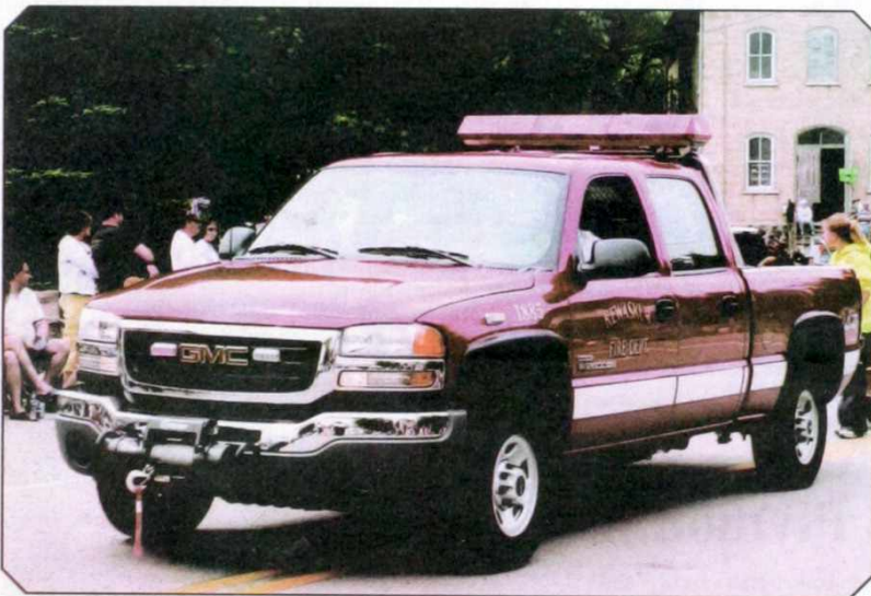
Jeff "Tubby" Boden proudly drives Kewaskum Fire Department's new brush fire truck. The 2005 GMC Duramax Diesel crewcab was put into service this past spring. Assistant Chief Mark Herges says the truck has a special feature that makes it able to draft water for filling tankers. This truck replaces a 1977 Chevrolet that has been sold.
