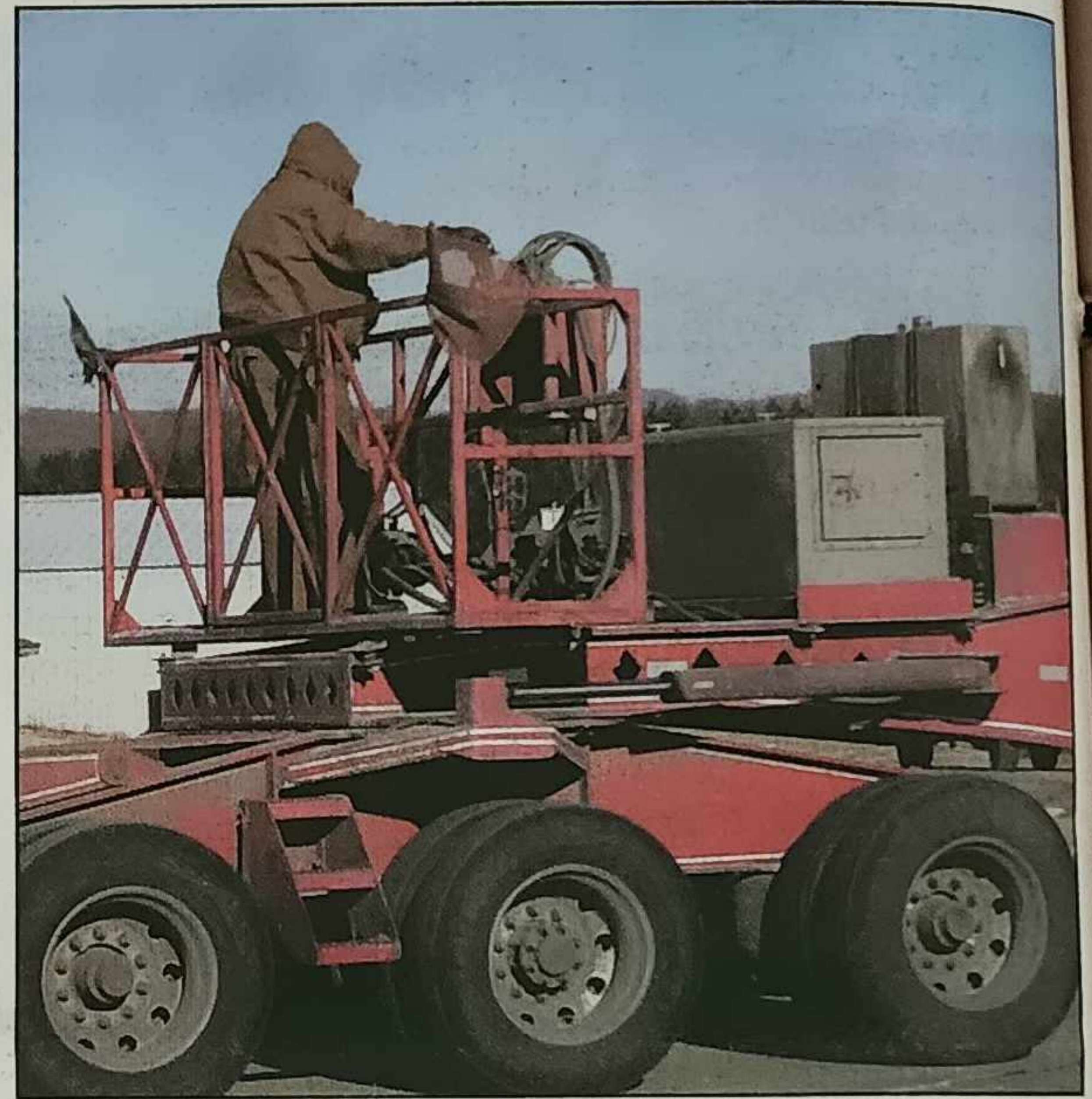
A cold job for one of the drivers of the rig. This person controlled the rear of the 20 axle trailer.
