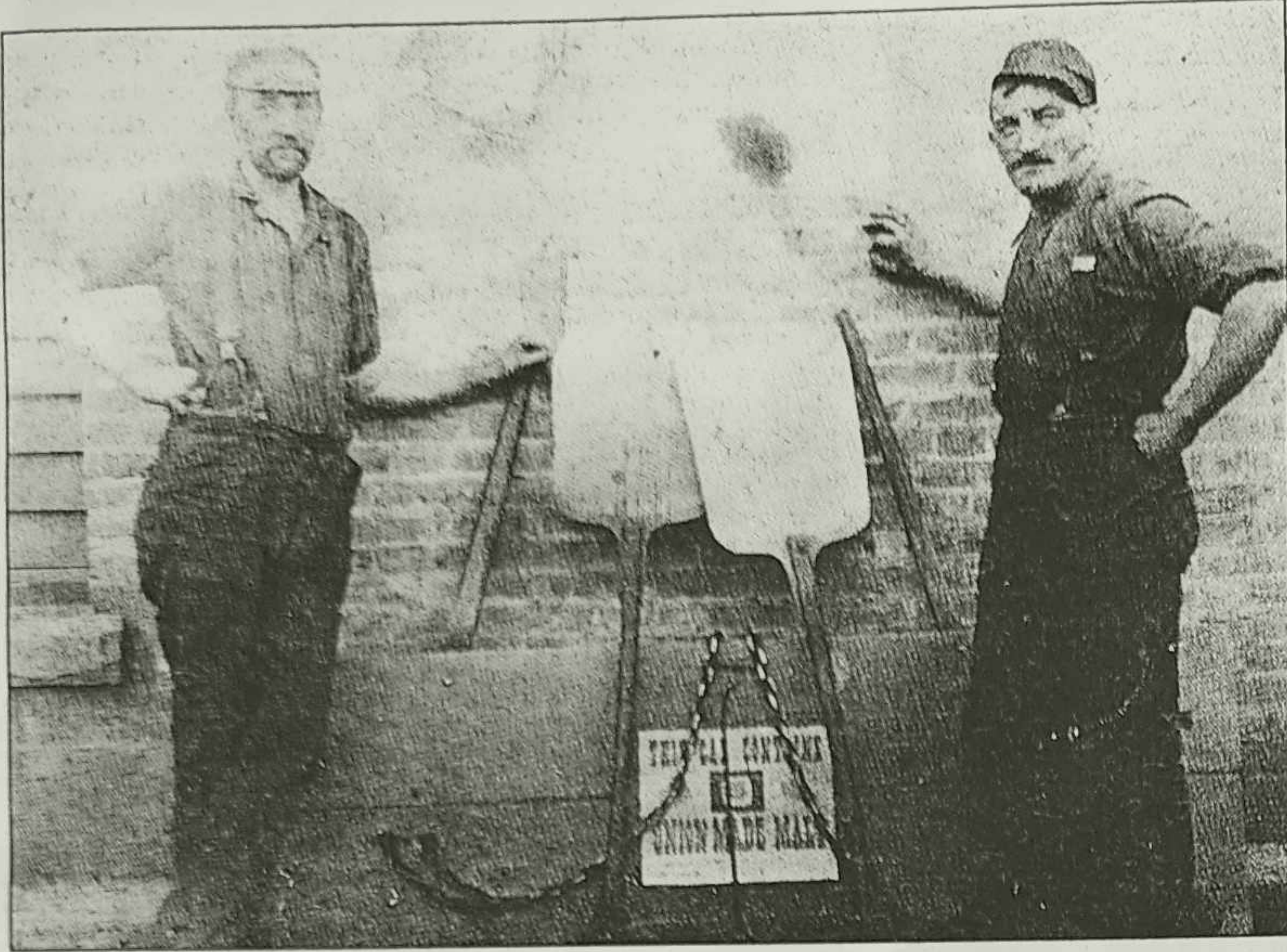
August Groeschel, right, and a co-worker, ca. 1912, at the Duluth Brewing Company. Although the brewery billed itself as "modern in every respect," maltsters still used the traditional tools of malting - large, flat shovels.
