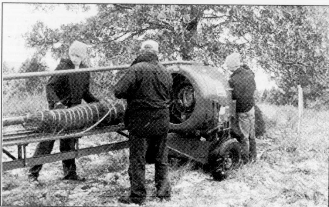
Crew members at Schroeder's Evergreens "bale" or wrap Christmas trees. Trees are baled so that they can be easily staked and loaded for shipping. Wisconsin Christmas tree growers harvest more than 3 million trees each year. More than 2 million are shipped to tree lots around the country. For more information contact the Wisconsin Christmas Tree producers Association at (608) 635-7735 or email at info@christmastrees-wi.org
