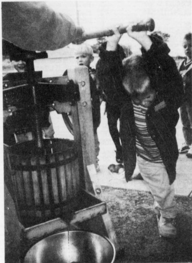
As you can see, turning the screw to press the apple bits is hard work!
