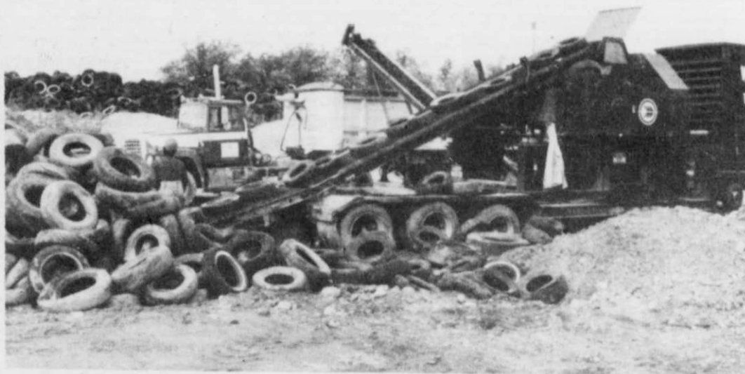
Employees of Waste Management of Wisconsin loaded tires onto a conveyor to be shredded and hauled to a Franklin landfill.
