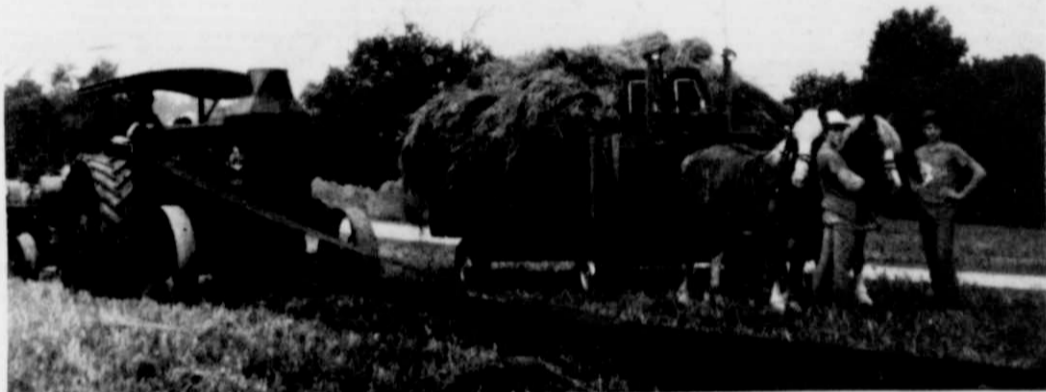
The 1921 LaPort Rumely oil tractor of Marshall Reysen provided power to drive the threshing machine's belt. A loaded wagon waited its turn to pull up to the thresher.
