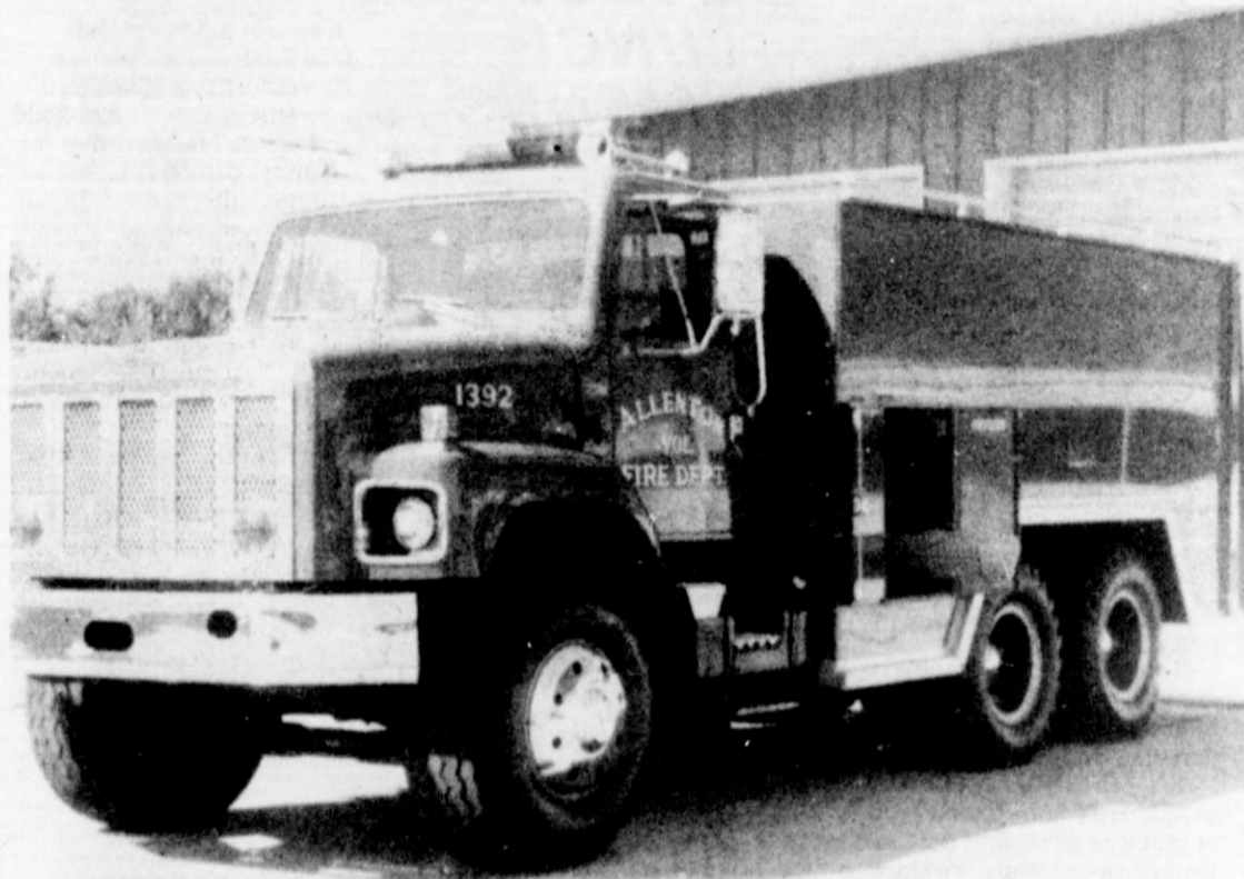
The Allenton Fire Department recently put their new tank truck into service. This truck features a 1984 International chassis bought from Cooleys, Inc. of West Bend. The truck is powered by a 350 hp. Detroit diesel engine and has an Allison automatic transmission. The body portion features a 3000 gallon tank which dumps its water in 90 seconds and can be filled in 2 1/2 minutes. The body was built by Welch Body of Marion, WI. and sold by General Fire Equipment of Oshkosh. Through the Washington County mutual aid pact this unit is available for assistance to all neighboring fire departments.
