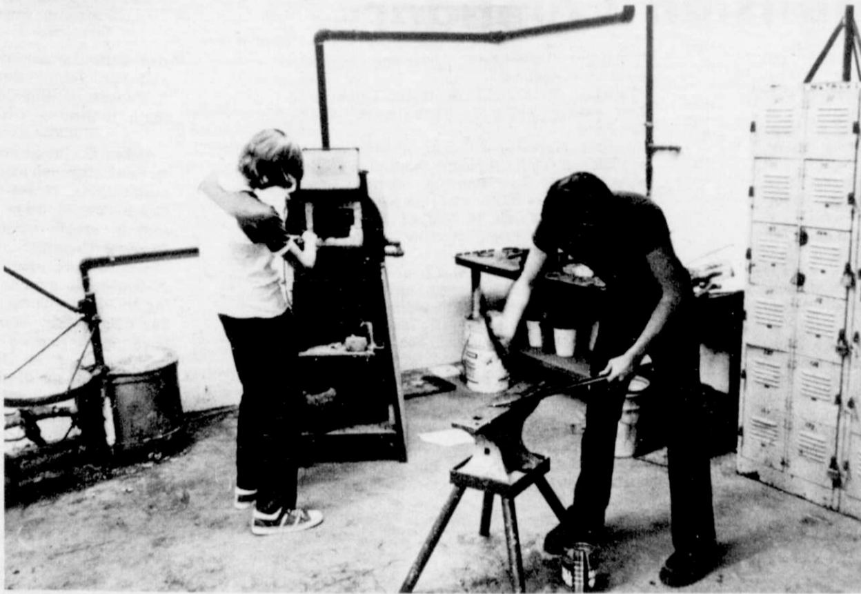
Forging a cold chisel is one of the required assignments in Metals I. Jim Haack (right) and Scott Klein (left) are developing their skills in this industrial arts area.
