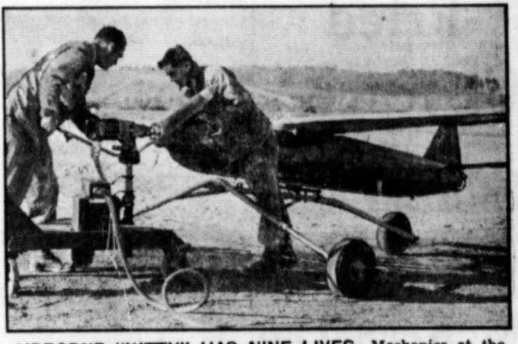
AIRBORNE "KITTY" HAS NINE LIVES—Mechanics at the U. S. Army's training grounds near Grafenwoehr, Germany, work on an "R-Cat" target plane which is used to tow targets during gunnery practice. Though often shot down, the sturdy craft are often repairable, and are used over and over again.
