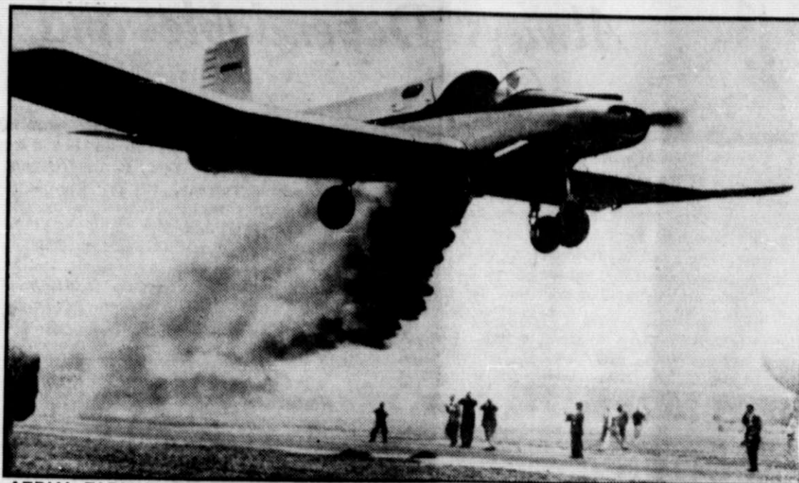
AERIAL FARMHAND —Swooping low to show off its crop-dusting ability, the "Fletcher Utility" goes through its paces at Rosemond, Calif. It is said by its manufacturers to be the first plane specifically designed for farm work to be put into volume production. Of all-metal construction, and with a 42-foot wingspan, the aerial workhorse is designed to pick up a 1250-pound load from an 870-foot, unimproved flight strip.
