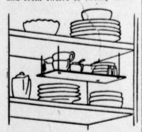
long. Make them from Masonite quarter-inch tempered hardboard. Insert long L-shaped hooks through drilled holes in the hardboard and then screw them into the shelf above. The hooks should be near the edges and at the corners of a shelf which is not longer than one foot. Intermediate hooks inserted mid-way on the long sides of the rectangle should be used if
