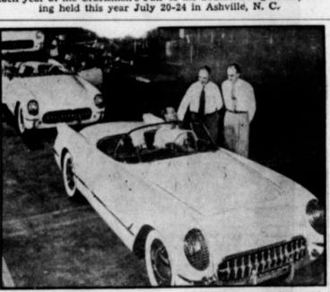
SOMETHING NEW-The "Corvette," the first automobile with a plastic body ever built by mass production methods, rolled off an assembly line last month at the Chevrolet plant in Flint, Mich.
