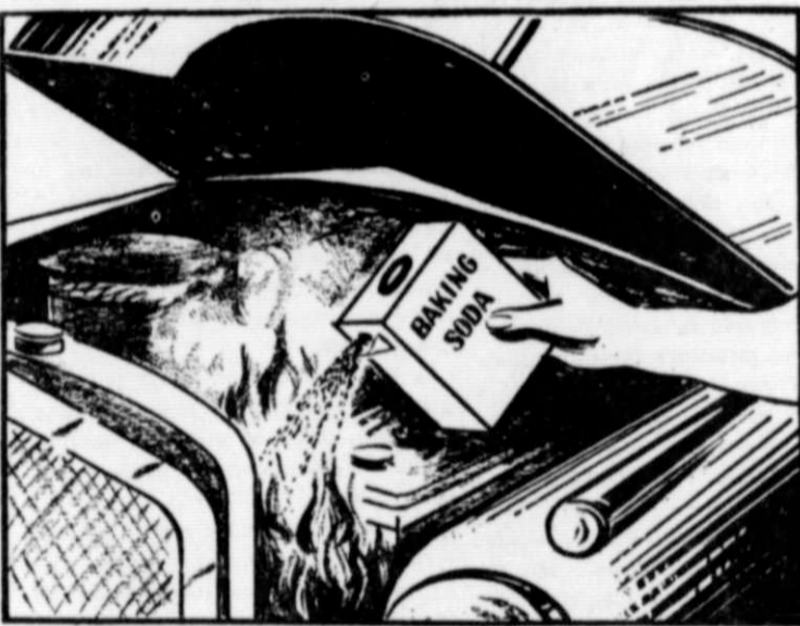
A pound of baking soda kept in the glove compartment of your car is a wise precaution. Fires can get started quickly—in the engine, even in the upholstery or ashtray. Sprinkle soda over the smoking spot, and fire will be instantly extinguished. Baking soda produces carbon dioxide which settles around the blaze, cuts off its oxygen, and squelches the fire.
