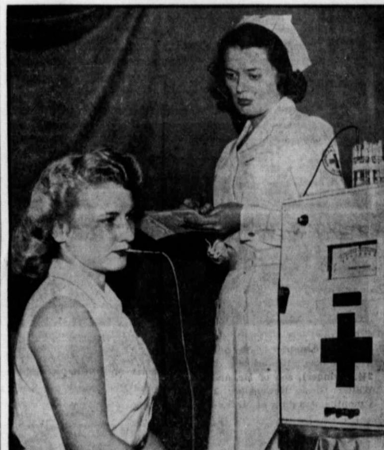
ELECTRONIC TEMPERATURE TAKER —A newly developed electronic thermometer takes temperatures twice as accurately as the old fashioned thermometer and 60 times as fast. Waiting the few seconds necessary to take a reading is pretty blond Philadelphia blood donor, Ariene Delaney. Ready to write the figure down is Red Cross Nurse Mary Douglas. Developed by Minneapolis-Honeywell engineers, the device will speed up blood donation time in case of disaster when many donations must be taken quickly.
