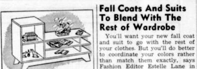
This combination table is easy to build with Handy Panels, the new stock small sizes of plywood now available at most retail lumber yards. Plans can be obtained by writing Douglas Fir Plywood Association, Tacoma 2, Wash.
