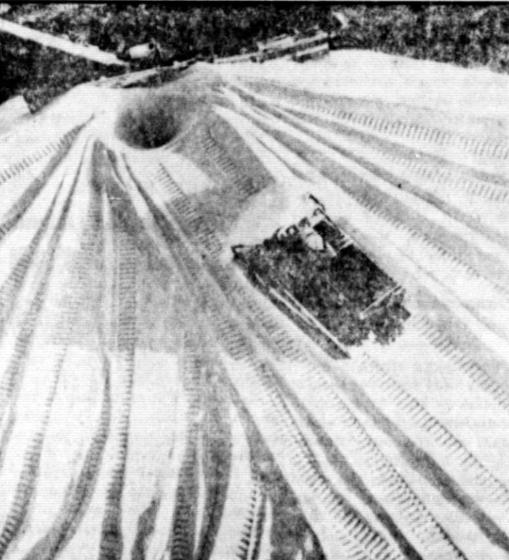
UP THE HILL TO YOUR TABLE —Cutting a swath along the rise a caterpillar tractor pushes salt to the loading pit in Baumberg, Calif. The salt pile is the result of sea water's being pumped into a diked area and evaporated.
