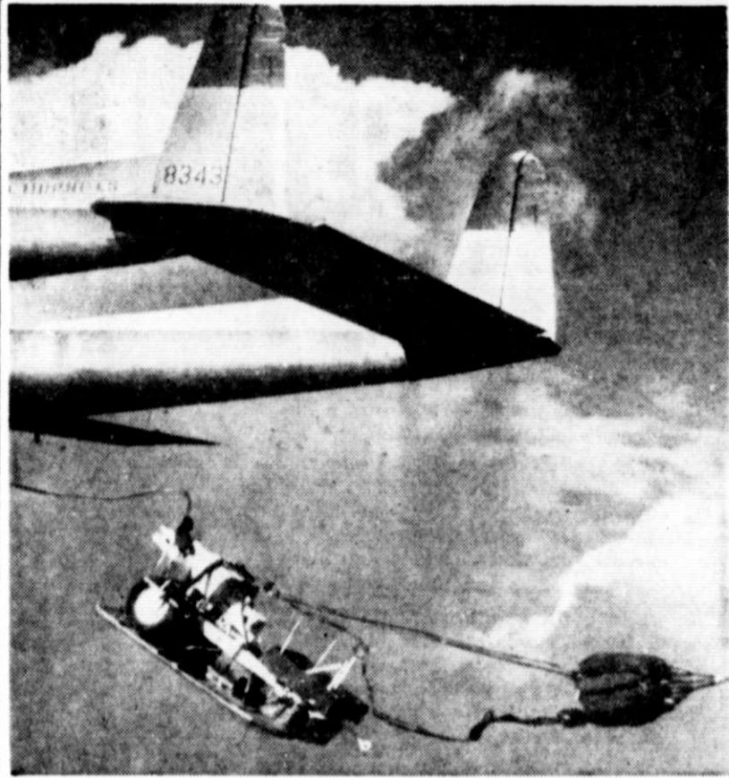
PLANE DROPS HOWITZER . . . United Nations ground forces in Korea which find themselves in a tight spot can request delivery by air of practically any weapon they might need. Here is a 105MM howitzer being released from a C-119 flying boxcar. Attached to three 100-foot parachutes the 5,000-pound artillery weapon will be gently lowered to the earth where the United Nations troops calling for it will be waiting to put it to use against the Chinese Red forces they face.
