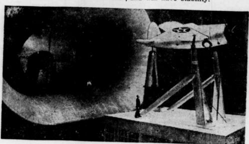
A FIGHTER PLANE, the Brewster XF2A-1, is shown mounted on struts in the full scale wind tunnel, ready for testing. The struts are convarious stresses which the plane undergoes in this largest wind tunnel in the world. (All pictures are official photographs released by the National Advisory Committee for Aeronautics.)
