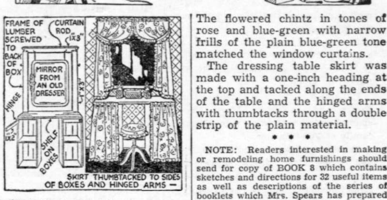
The illustration shows what became of a mirror and piano stool. To the mirror and stool were added two wooden boxes from the grocery. These were placed on end about 18 inches apart and a shelf of half-inch plywood was screwed to the top. A frame was then screwed to the back of the boxes as shown. A curtain rod was placed across the top and the mirror hung lengthwise under it. An arm was then hinged to the front of each box. White, because white furniture is smart and because it matched the woodwork.
