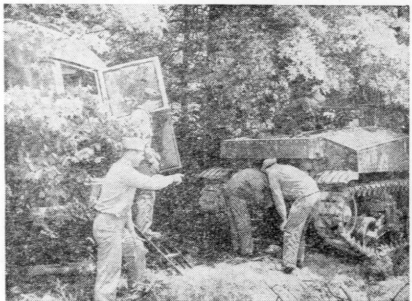
An ordnance maintenance officer directs repair of the tank in a camouflaged position in the "combat" zone. The machine shop on wheels carries the tools, machinery and spare parts needed for repair.
