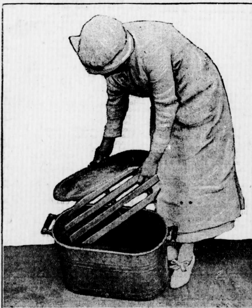
Homemade Hot Water Bath Sterilizing Outfit, Showing Satisfactory Type of Wooden False Bottom.
