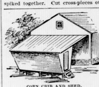
CORN CRIB AND SHED. of 2x4 stuff; run over on shed so as to form shelf (see cut). This will be very handy in getting corn out of crib. Next cut studding to length, using 2x6 stuff, placed two feet on centers. Put on A lady said: "The first time I drank roofing strips, 1x6 stuff; place two feet sheet steel roofing, which will be found cheaper for this kind of building. Any farmer can build it with the following
