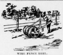
wire, one end is stapled to the barrel the dirt and so does not gather much litter. If it is a temporary fence, it is frequently necessary to move it but a ed all the way, but if the removal is to a greater distance, the rod can be taken out and the barrel with its coil of wire lifted into a wagon.-Orange Judd
