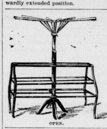
Plyotally connected to the central ost are also folding frames with horizontal bars, forming a clothes horse or rack at each side for supporting large pieces of clothing. Each side frame is independent of the other, so that either one or both of them may be used at a time or both of them may be hooked
